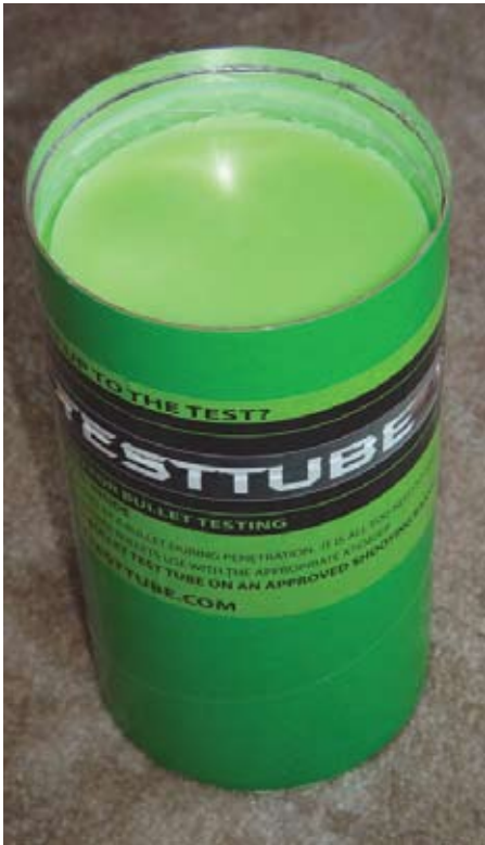
Ballistic Technology's Bullet Test Tube is essentially a tube filled with a wax-type penetration medium.
