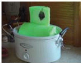
A 6-quart crockpot works well to melt the Bullet Test Tube medium in order for it to be recycled.
