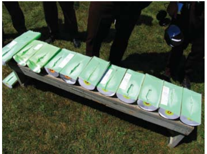
Testing conducted by Ballistic Technology for the Department of Natural Resources demonstrated the differences between various .223 ammunition. (Image supplied by Ballistic Technology.)
